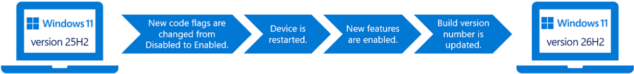
Figure 3. The four stages of an update from one version to another: New code flags change from Disabled to Enabled, device is rebooted, new features are enabled, and the Windows build version number is updated.
